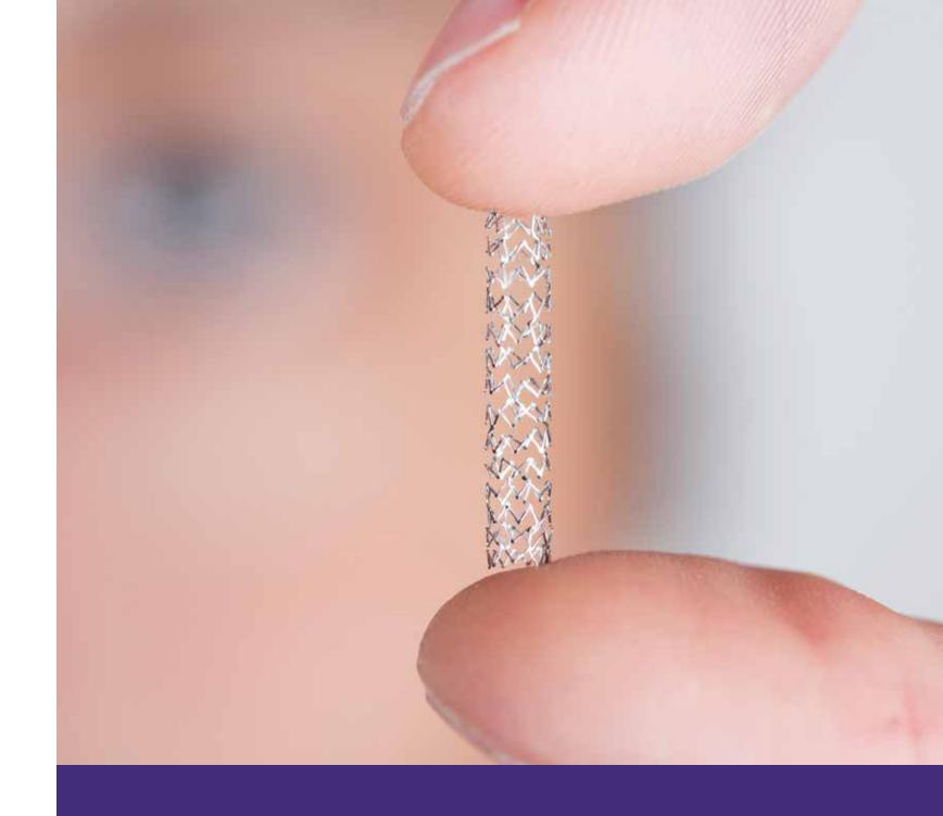
An advanced material like Nitinol possesses critical physical and mechanical properties and offers elegant solutions to meet complex anatomical and physiological needs. Nitinol's biocompatibility, kink resistance, superelasticity and ability to shape set, helps medical device
